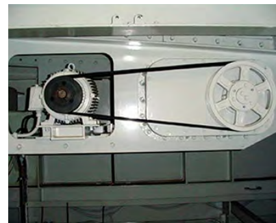
VGF Integral Motor Mount is mounted to the vibrator assembly.
